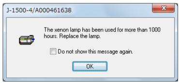
Figure 2.12 Warning message for xenon lamp usage time
