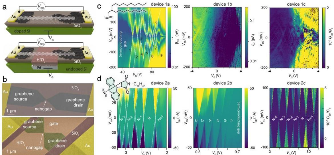
*Examples of single-electron quantum transport devices based on molecular graphene nanoribbons, fabricated and measured in my labs, showing the geometry of the fabrication (a), the actual devices (b), non-optimized transport (c), ultra-clean Coulomb blockade transport features optimized for quantum experiments (d).*
