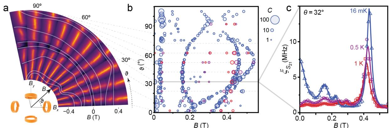
*Examples of strong coupling of a high quality resonator with a Gd(III)-based metal complex, at mK temperatures, showing the angular evolution of the avoided level*
