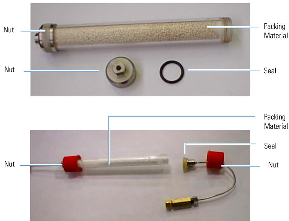
**Figure 8-13.** Preparation of the Adsorption Filters
