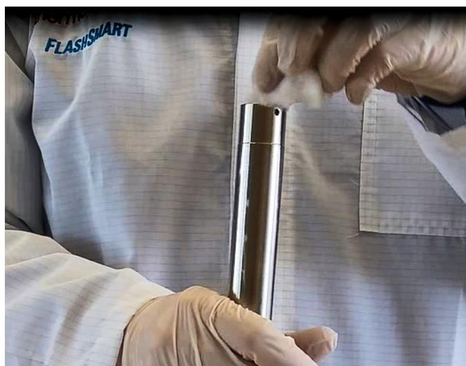
**Figure 8-8.** Introduction of Quartz Wool as Last Layer of the Sequence
