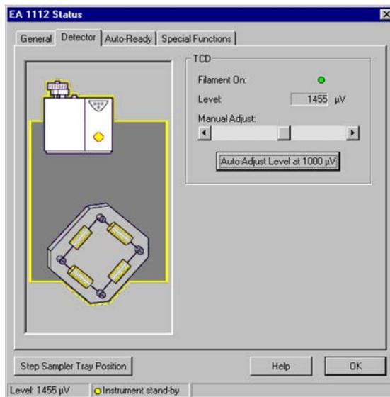
**Figure 11-11.** Detector Status Tab
