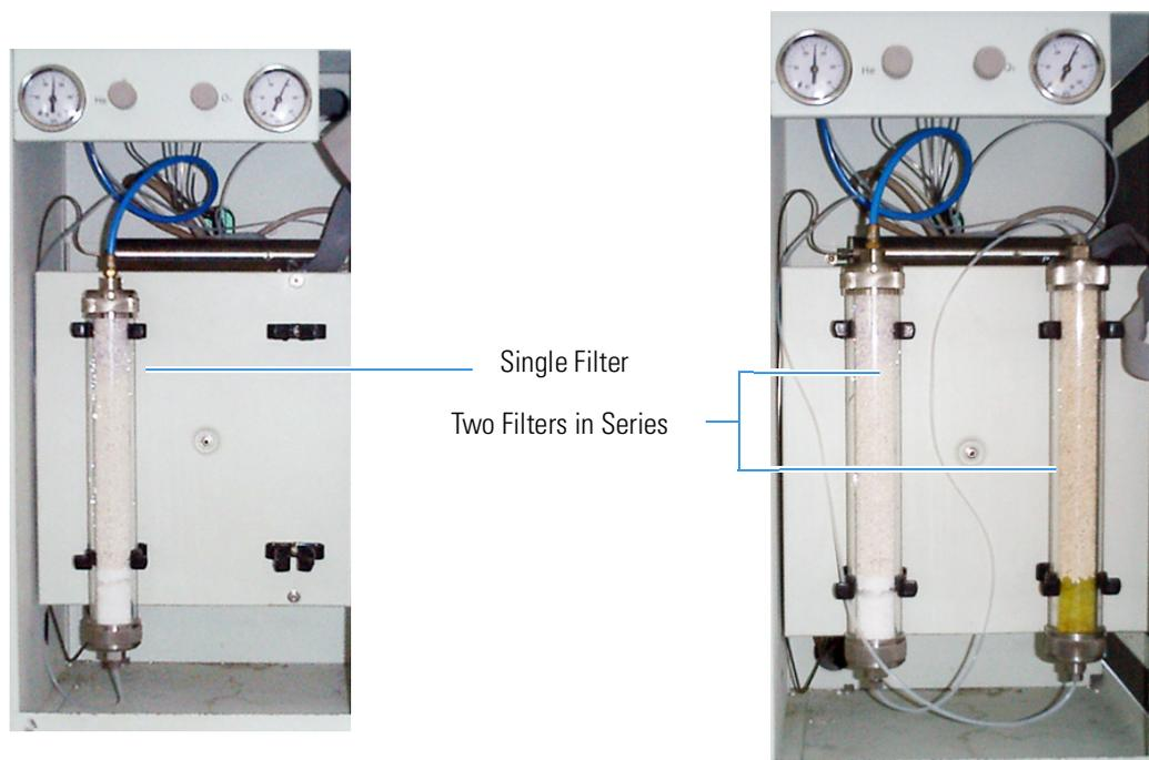
**Figure 9-14.** Adsorption Filters Installed in the Detector Compartment
