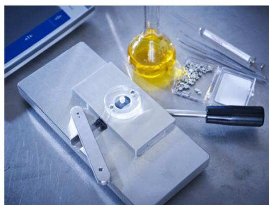
**Figure 10-7.** Accessories for Weighing Liquid Samples
