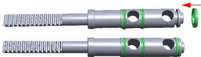
**Figure 14-20.** Inserting the third O-ring
