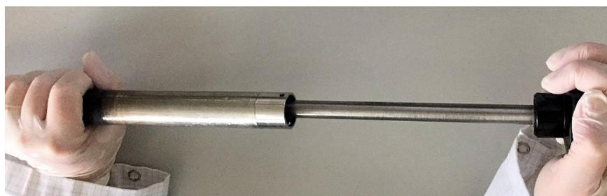
**Figure 14-1.** Removal of the Filling Material from an Alloy Steel Reactor
