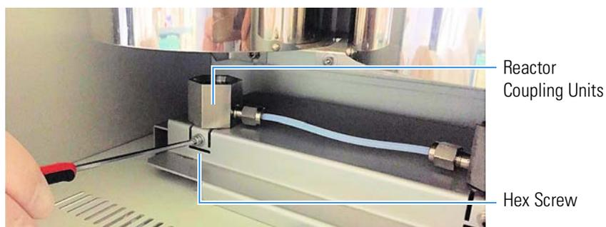
**Figure 14-6.** Removal of the Reactors Coupling Unions
