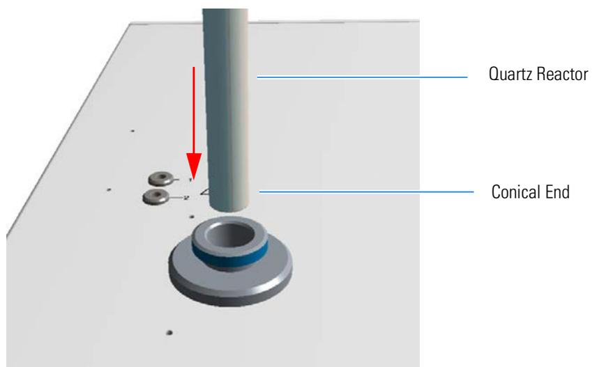
**Figure 9-2.** Introduction of the Quartz Reactor into the Furnace
