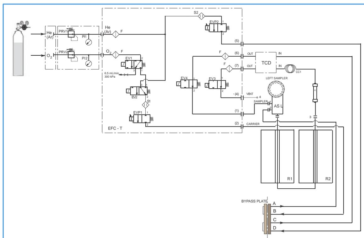
**Figure 4-21.** Instrument Parts Diagram and Pneumatic Diagram for NC Configuration
