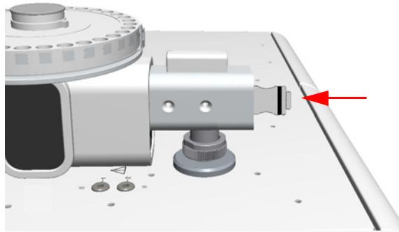
**Figure 14-14.** Reinstalling the Shaft (2)
