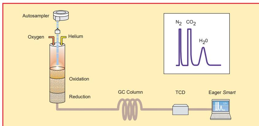
**Figure 4-4.** Schematic of CHN Configuration
