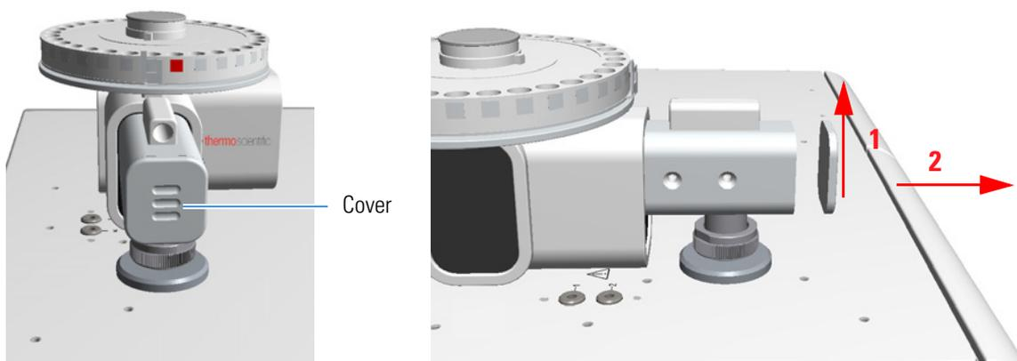
**Figure 14-10.** Removal of the MAS Plus Autosampler Cover
