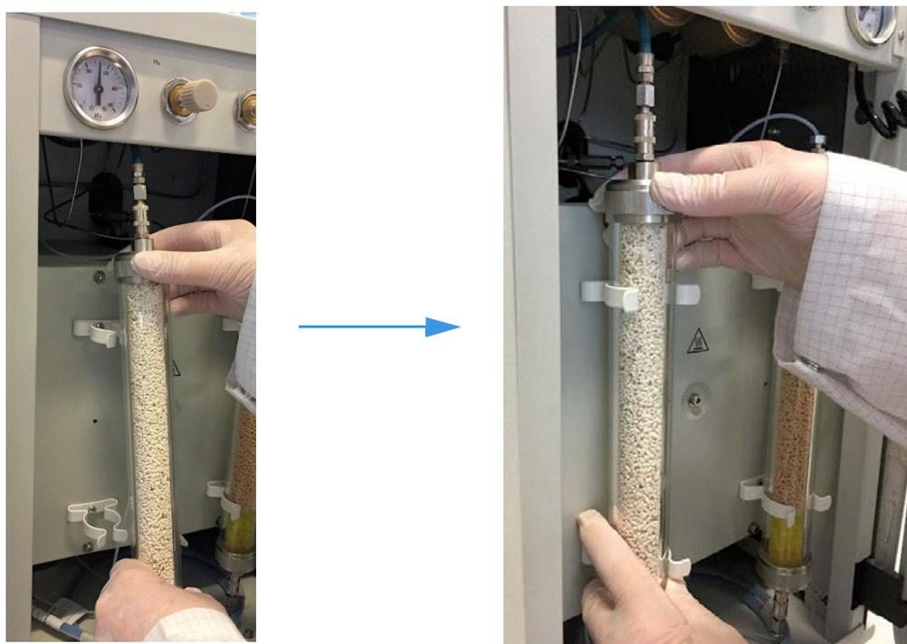
**Figure 9-16.** Installation of the Filters into the Detector Compartment
