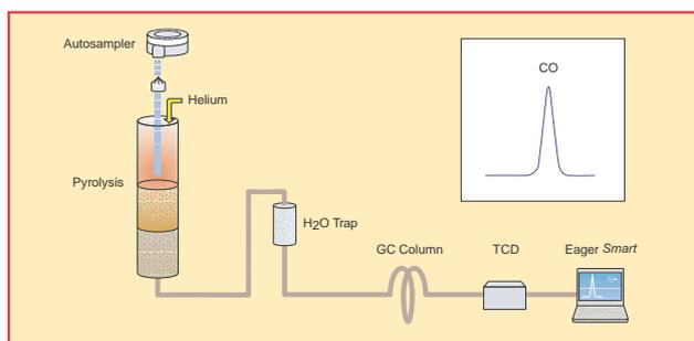
**Figure 4-14.** Schematic of CHNS/O Configuration (O Determination)
