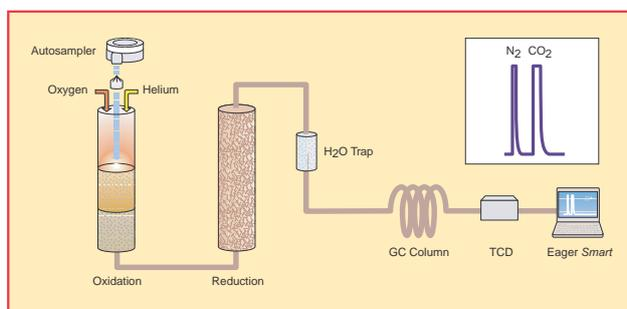
**Figure 4-26.** Schematic of NC Soils Configuration
