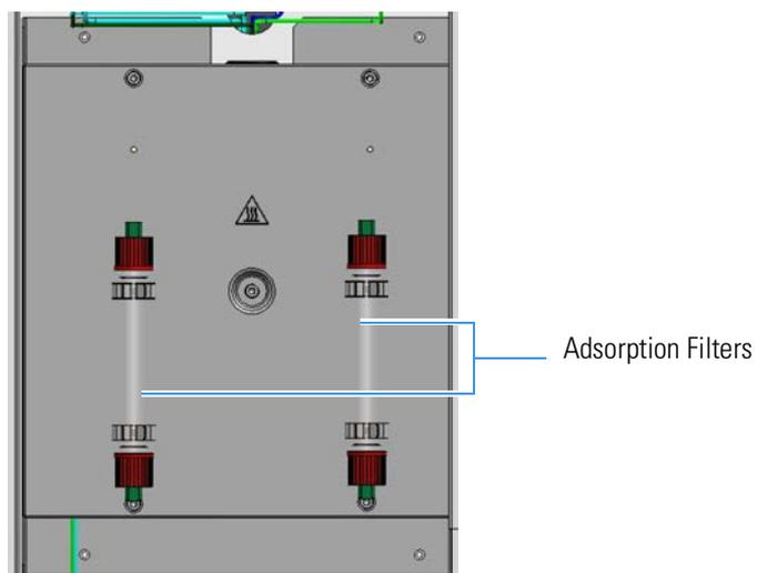
**Figure 3-10.** Adsorption Filters Installed
