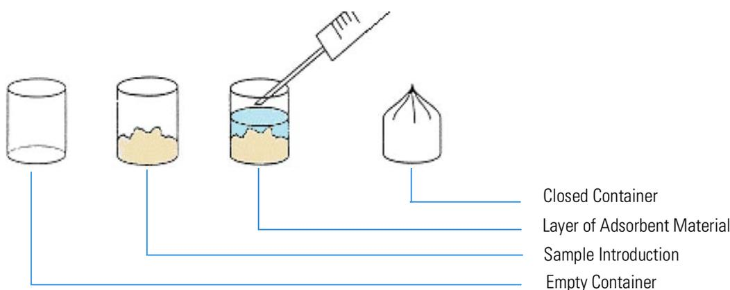
**Figure 10-10.** Weighing of a Liquid Sample Deposited on Adsorbent Material
