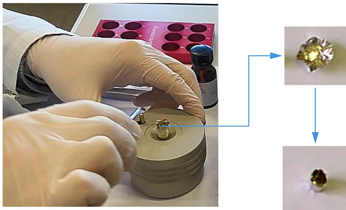
**Figure 10-3.** Preparation of the Tin Container (2)
