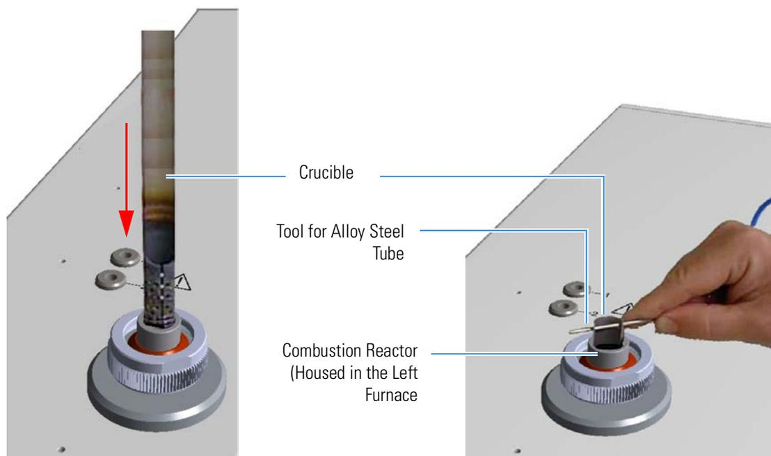
**Figure 9-10.** Introduction of the Crucible into the Combustion Reactor
