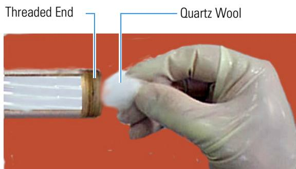
**Figure 8-11.** Introduction of Quartz Wool into the Tube
