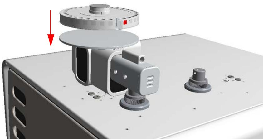
**Figure 6-8.** Placing the sample tray onto the toothed wheel
