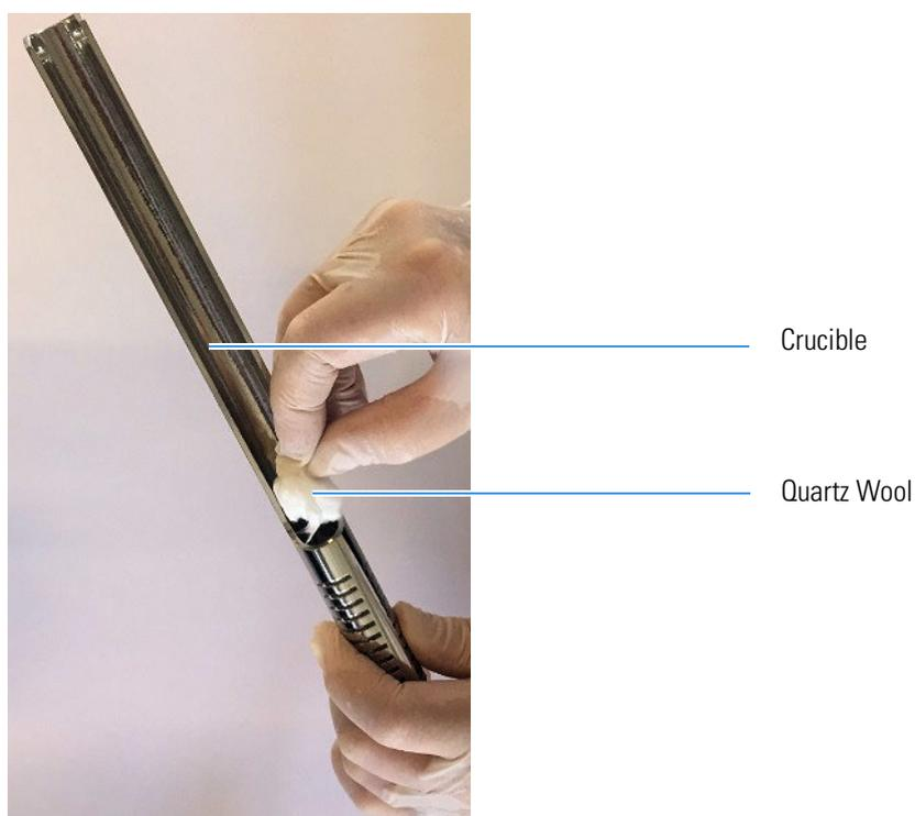
**Figure 8-9.** Introduction of Quartz Wool into the Crucible
