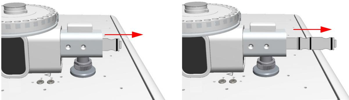
**Figure 14-11.** Removal of the Shaft
