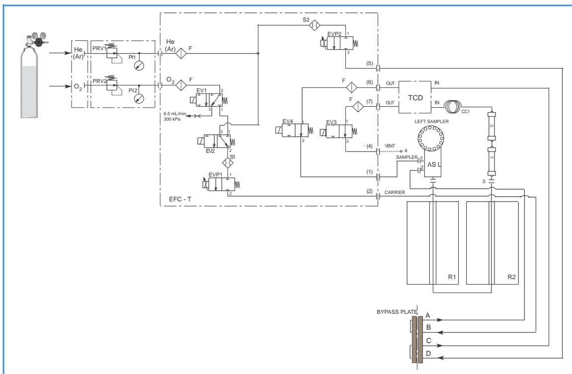
**Figure 4-19.** Instrument Parts Diagram and Pneumatic Diagram for N (Nitrogen) Configuration
