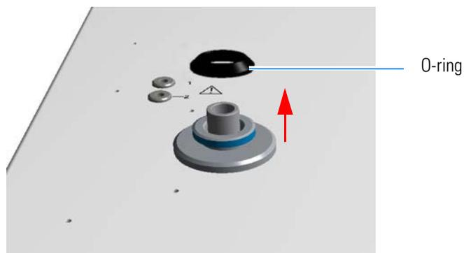
**Figure 9-19.** Removal of the Alloy Steel Reactor O-ring
