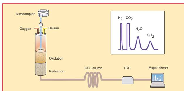
**Figure 4-13.** Schematic of CHNS/O Configuration (CHNS Determination)
