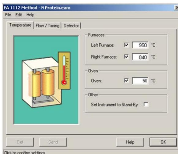
**Figure 11-7.** Example of Analyzer Parameters
