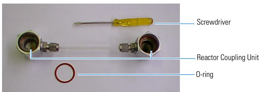
**Figure 14-7.** View of the Reactors Coupling Unions
