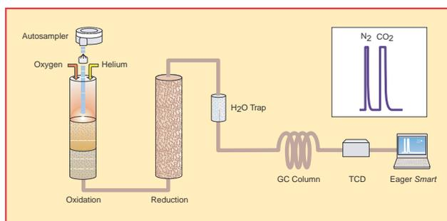
**Figure 4-22.** Schematic of NC Configuration
