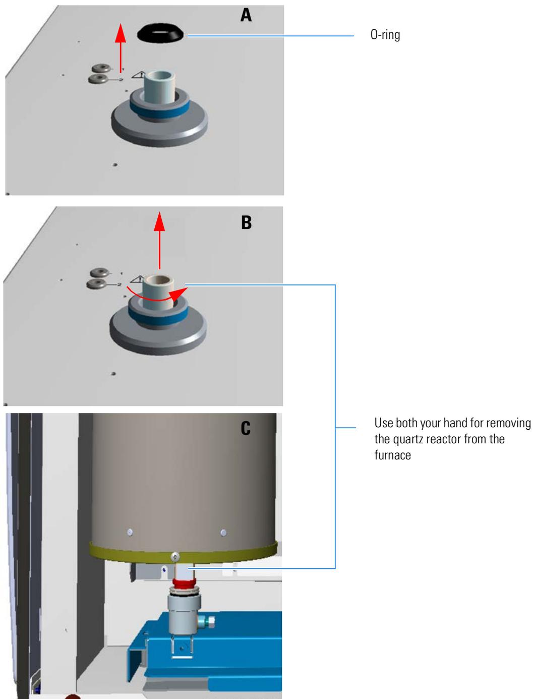
**Figure 9-17.** O-ring and removal of the quartz reactor from the furnace
