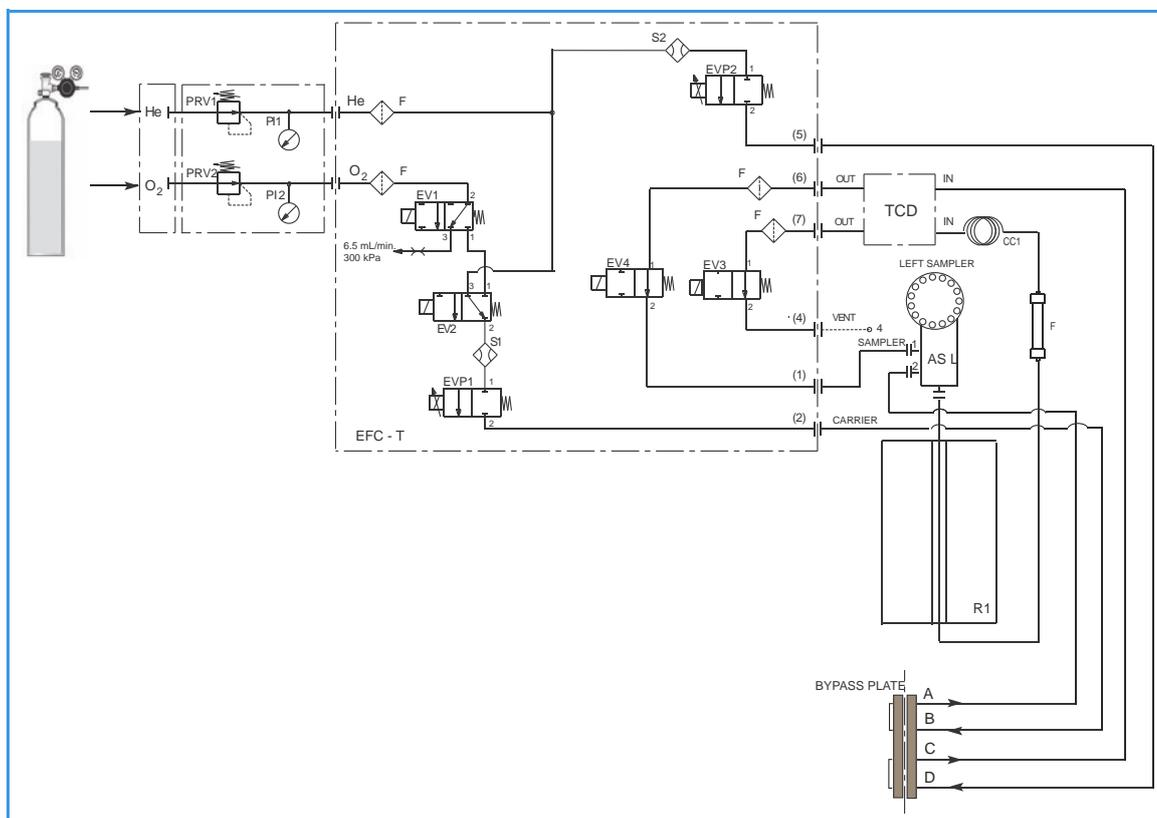
**Figure 4-23.** Instrument Parts Diagram and Pneumatic Diagram for NCS Configuration
