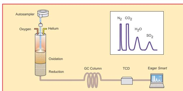
**Figure 4-10.** Schematic of CHNS Configuration
