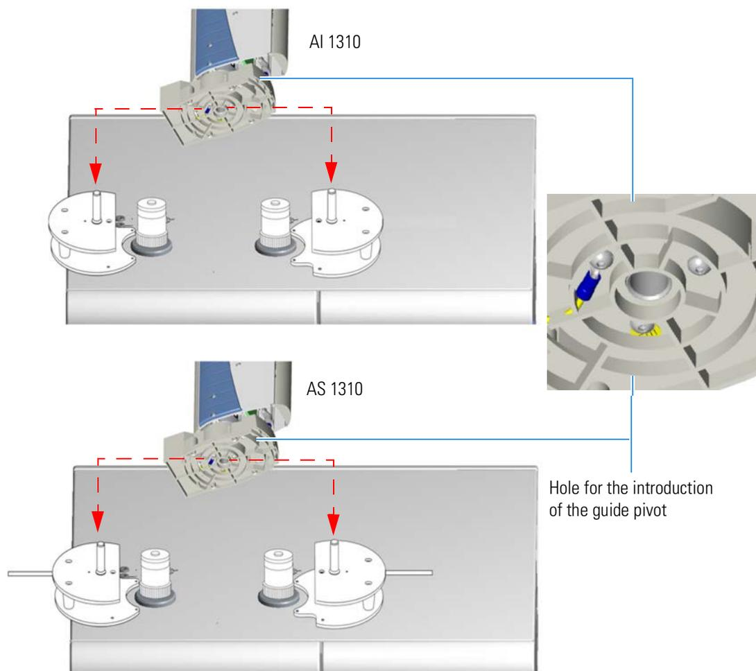
**Figure 7-10.** Installation of the Sampling Unit
