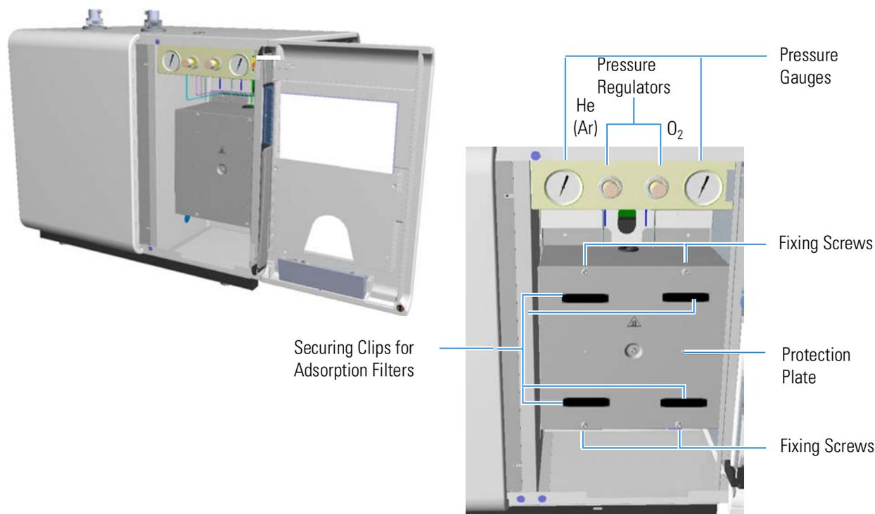
**Figure 3-9.** Oven Compartment Internal View
