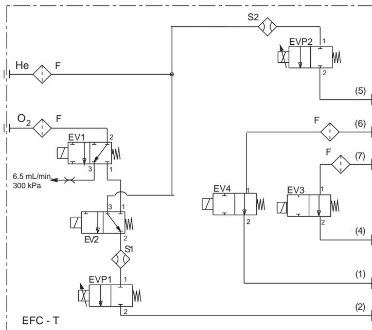
**Figure 4-2.** Thermo-regulated EFC-t Module for helium carrier gas
