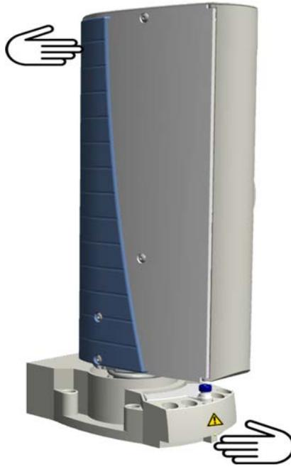
**Figure 7-1.** How to Lift and Carry the Sampling Unit
