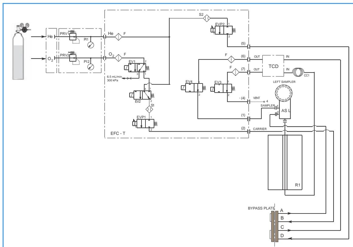
**Figure 4-3.** Instrument Parts Diagram and Pneumatic Diagram for CHN Configuration
