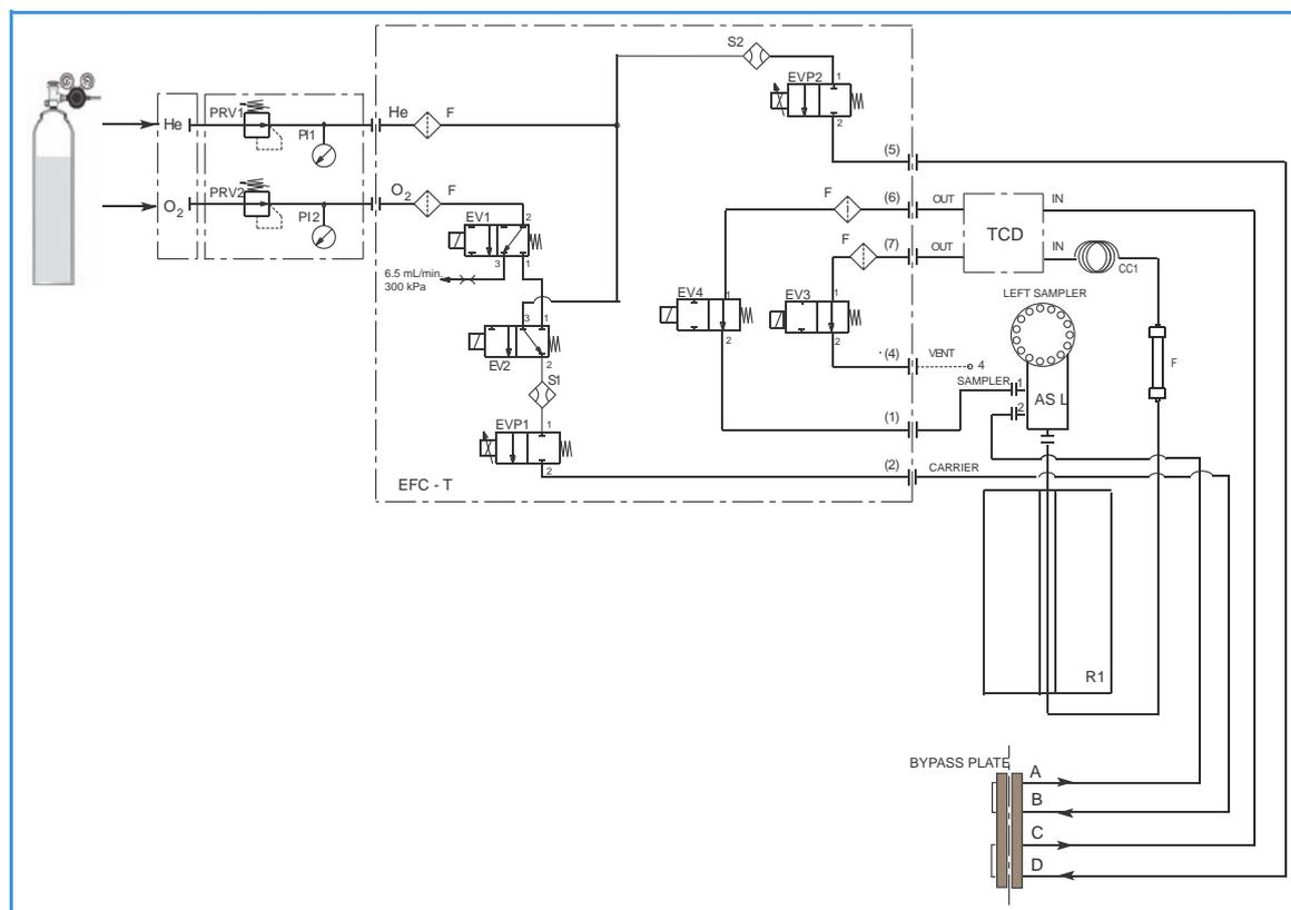
**Figure 4-15.** Instrument Parts Diagram and Pneumatic Diagram for S (Sulfur) Configuration
