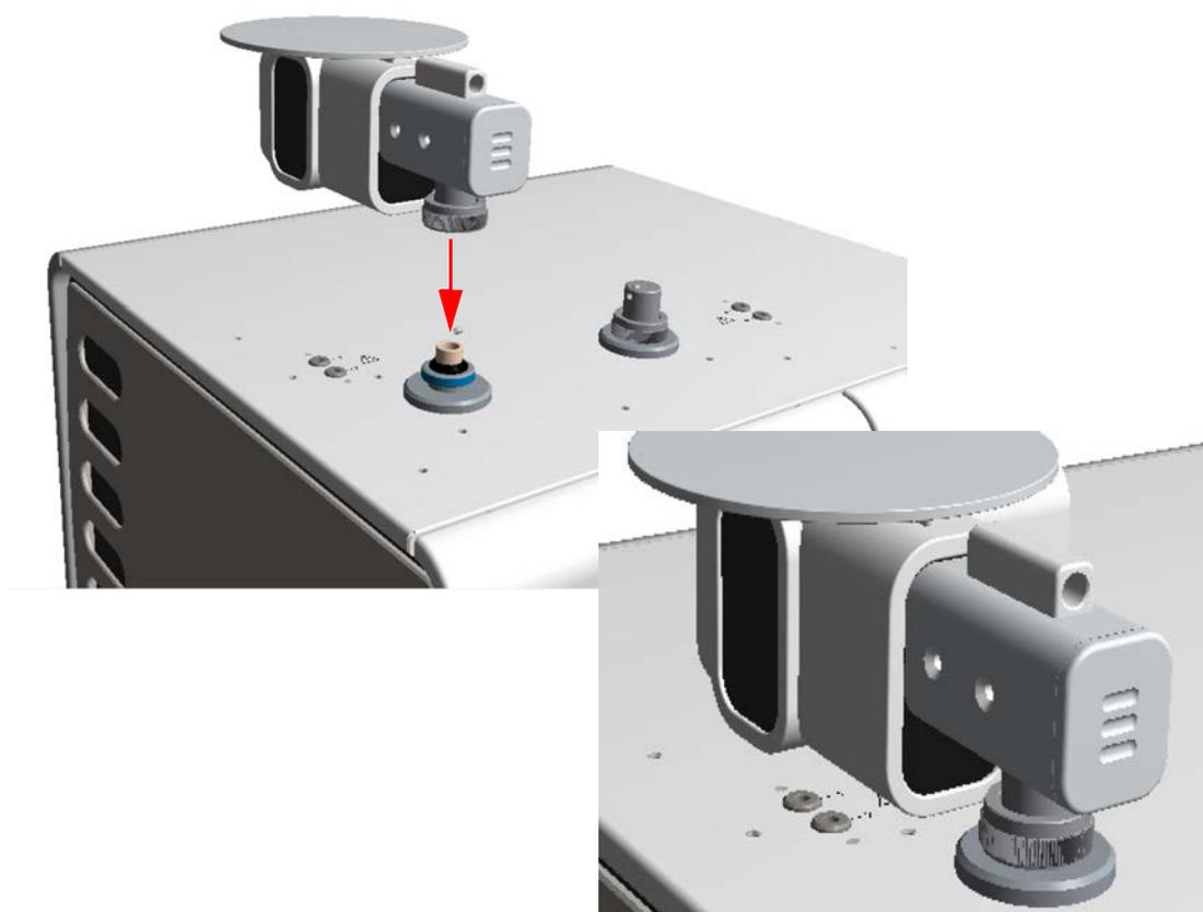
**Figure 6-6.** Installing a MAS autosampler
