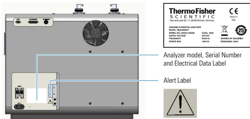
**Figure 2-3.** FlashSmart. rating plate (example)
