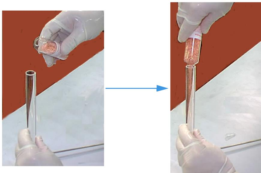
**Figure 8-3.** Filling of the Quartz Reactor
