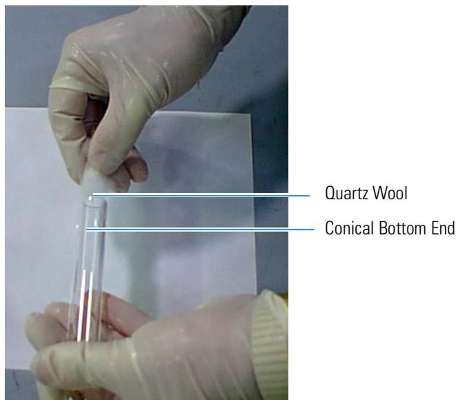
**Figure 8-1.** Introduction of Quartz Wool into the Conical End of the Reactor
