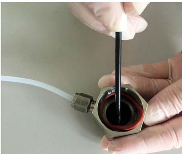
**Figure 14-9.** Introduction of the O-ring from the Coupling Union
