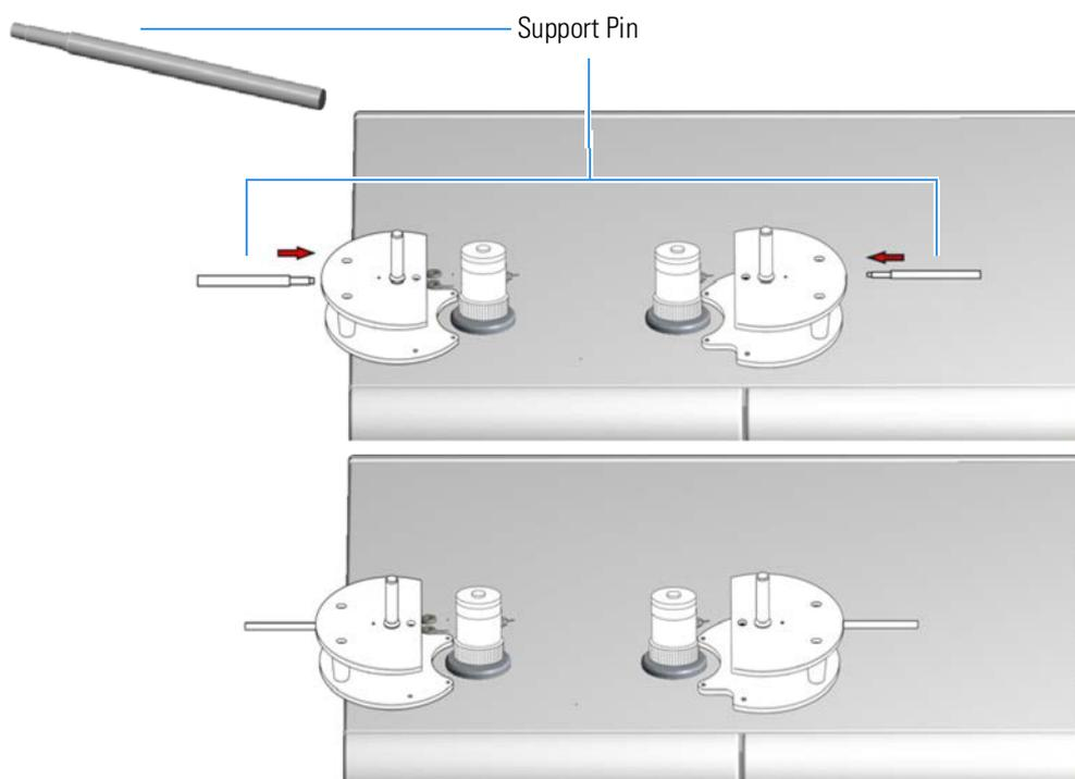
**Figure 7-8.** Mounting the Support Pin
