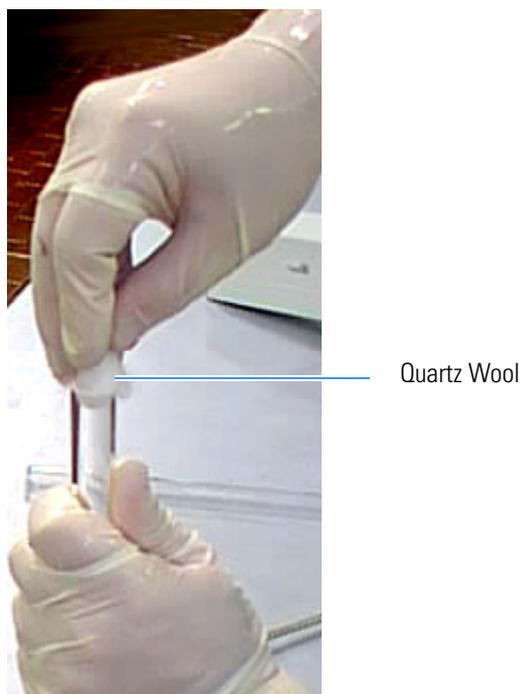
**Figure 8-4.** Introduction of Quartz Wool as Last Layer of the Sequence
