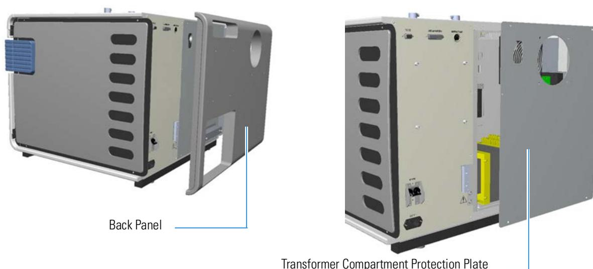
**Figure 3-18.** Accessing the Transformer Compartment
