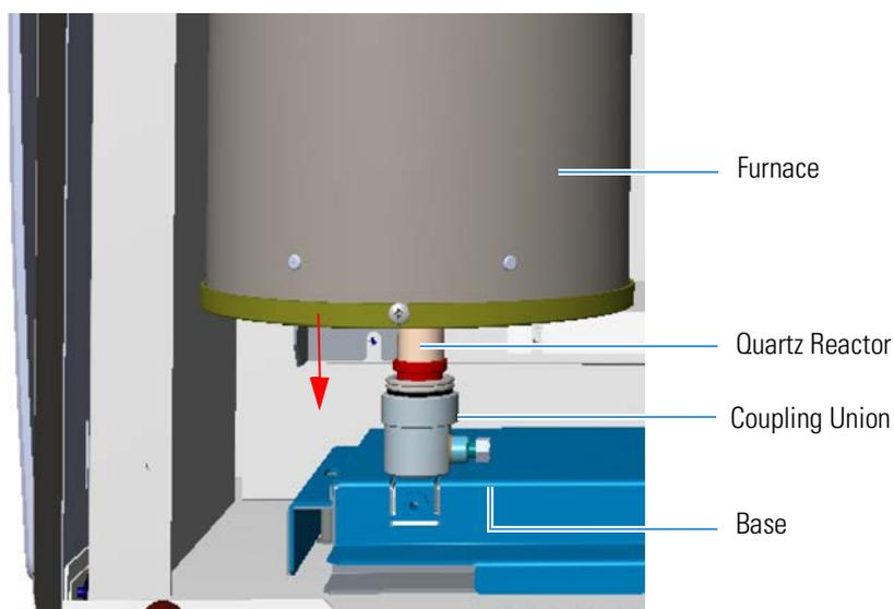
**Figure 9-3.** Driving the Reactor into the Furnace
