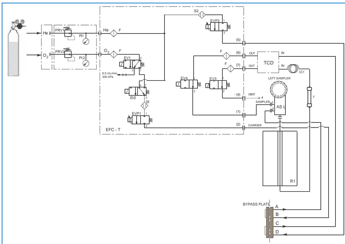
**Figure 4-17.** Instrument Parts Diagram and Pneumatic Diagram for O (Oxygen) Configuration
