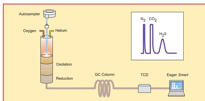
**Figure 4-7.** Schematic of CHN/O Configuration (CHN Determination)
