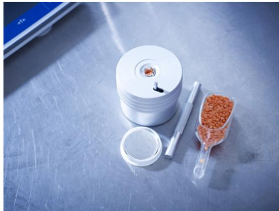
**Figure 10-1.** Accessories Required for Weighing Solid Samples
