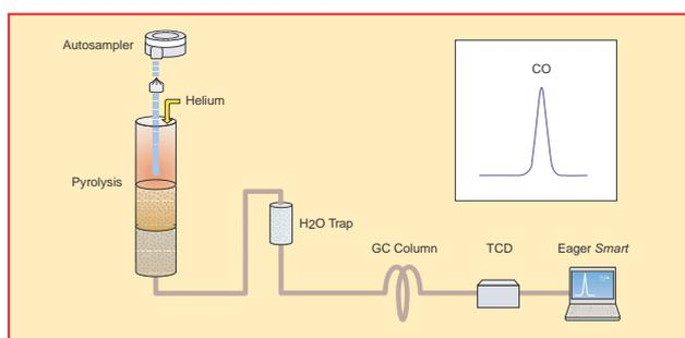
**Figure 4-8.** Schematic of CHN/O Configuration (O Determination)
