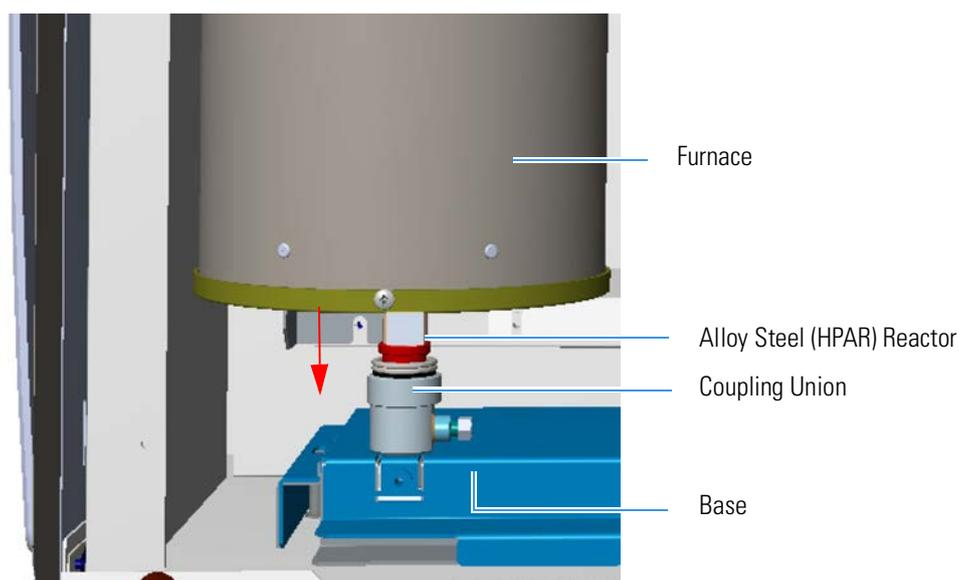
**Figure 9-7.** Driving the Reactor into the Furnace
