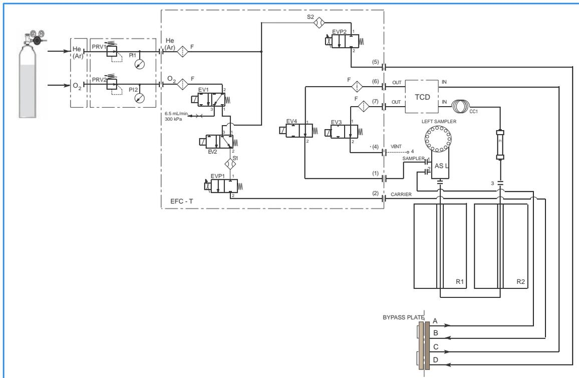
**Figure 4-25.** Instrument Parts Diagram and Pneumatic Diagram for NC-Soils Configurations
