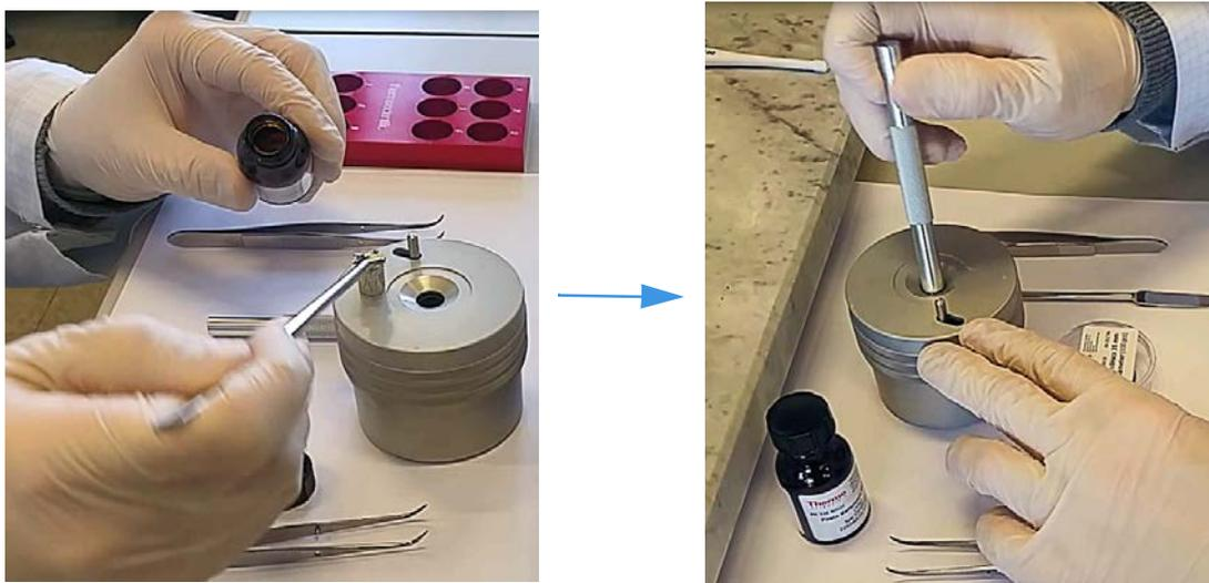
**Figure 10-4.** Introduction and Compression of the Sample
