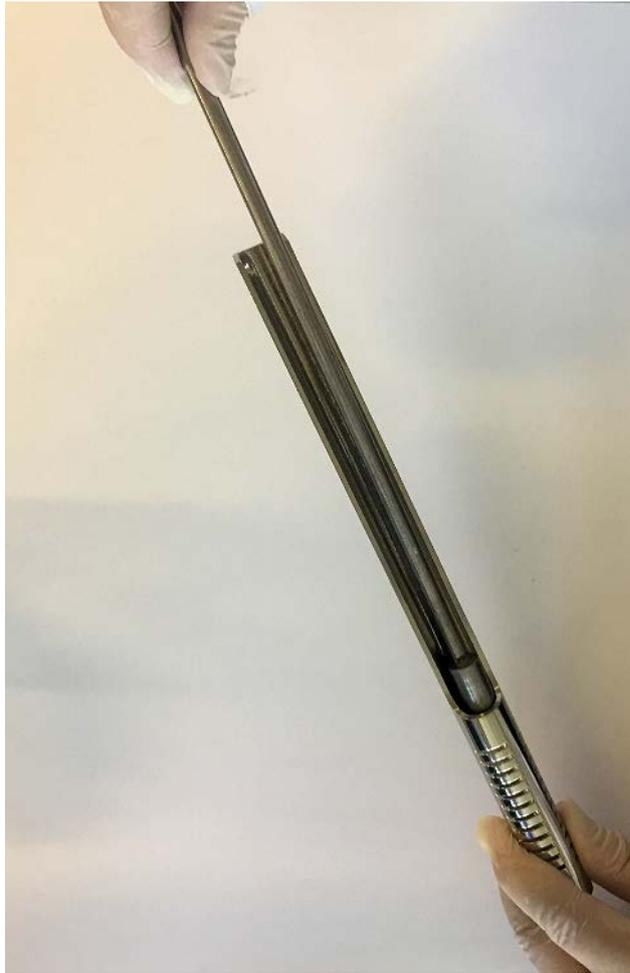
**Figure 8-10.** Compression of Quartz Wool into the Crucible
