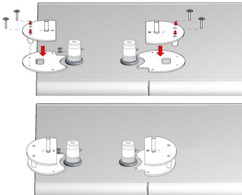
**Figure 7-7.** Mounting Sampler Support
