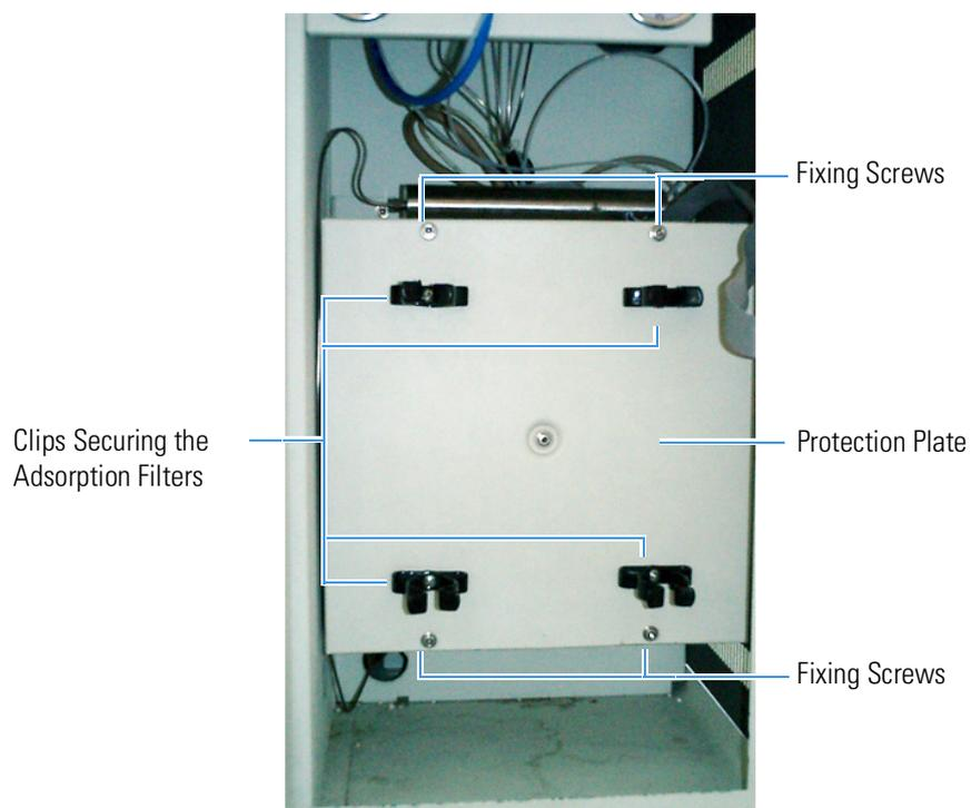
**Figure 14-4.** Access to the Detector
