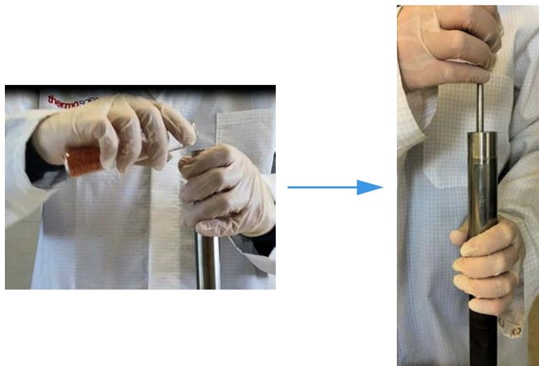
**Figure 8-7.** Filling of the Alloy Steel (HPAR) Reactor and Compression of Materials
