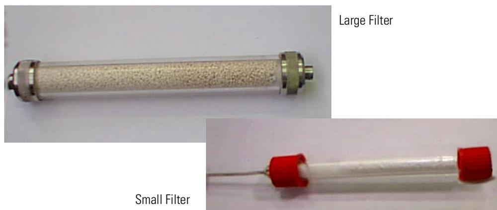
**Figure 8-14.** Result of the Filling of a Large and Small Adsorption Filter
