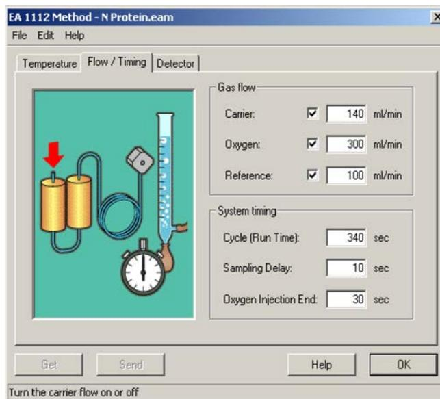
**Figure 12-2.** Flow Timing Tag
