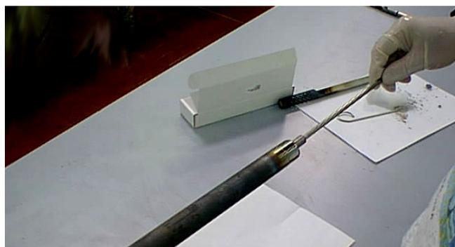
**Figure 8-6.** Compression of Quartz Wool into the Alloy Steel (HPAR) Reactor
