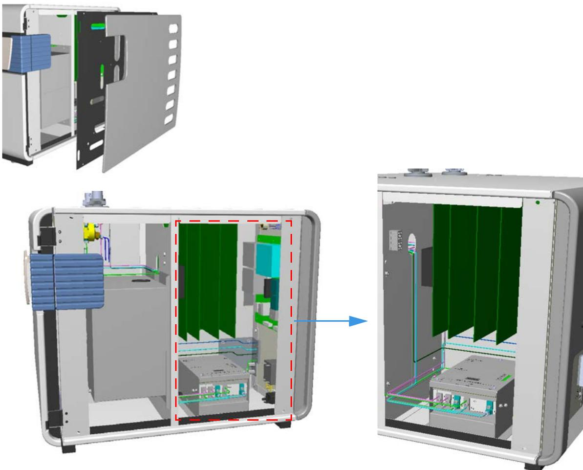
**Figure 3-13.** Electrical Compartment Internal View
