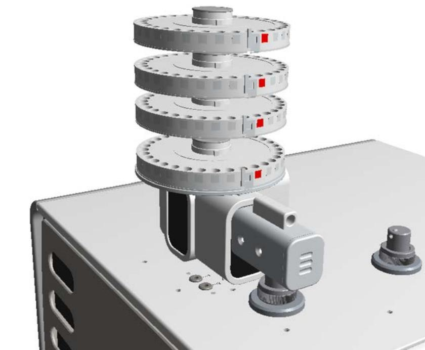
**Figure 6-9.** Installing additional sample trays
