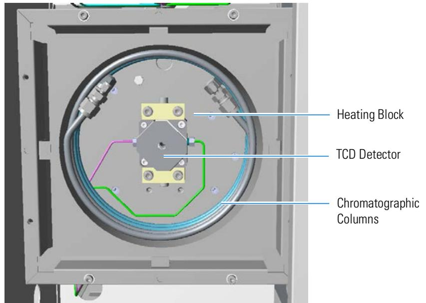
**Figure 3-12.** Thermostatic Chamber Internal View
