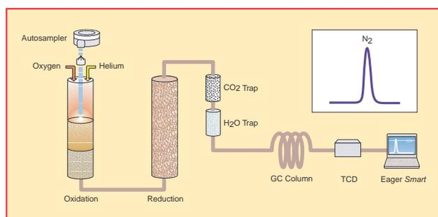
**Figure 4-20.** Schematic of N Configuration
