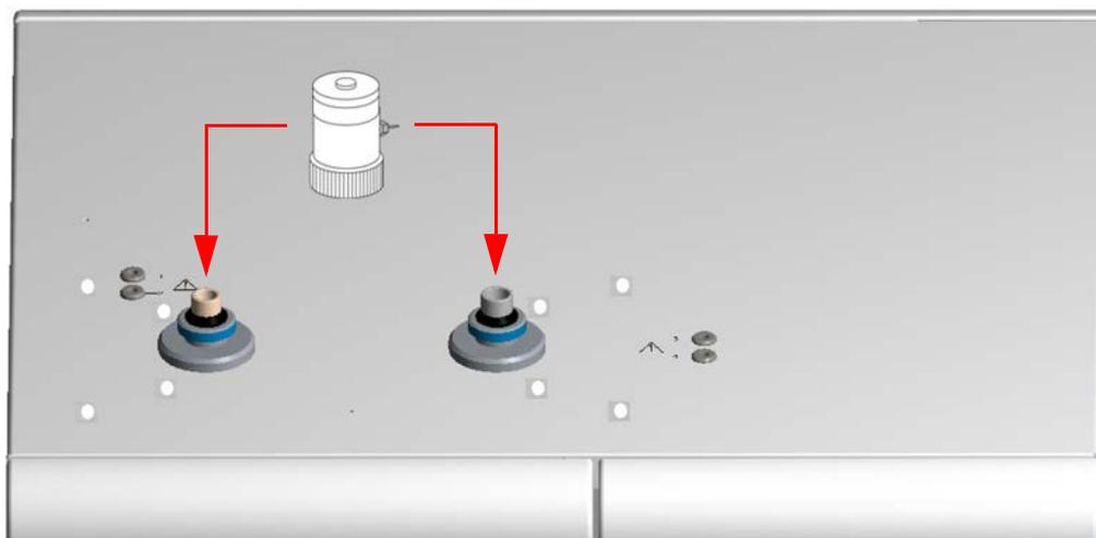
**Figure 7-3.** Direct Injection Device Installation
