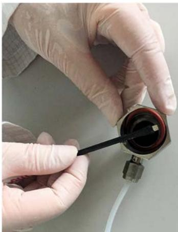
**Figure 14-8.** Removal of the O-ring from the Coupling Union
