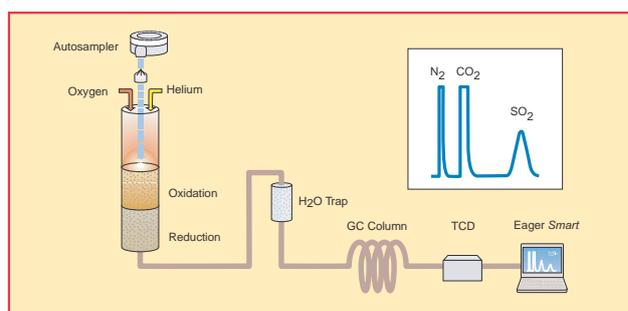
**Figure 4-24.** Schematic of NCS Configuration
