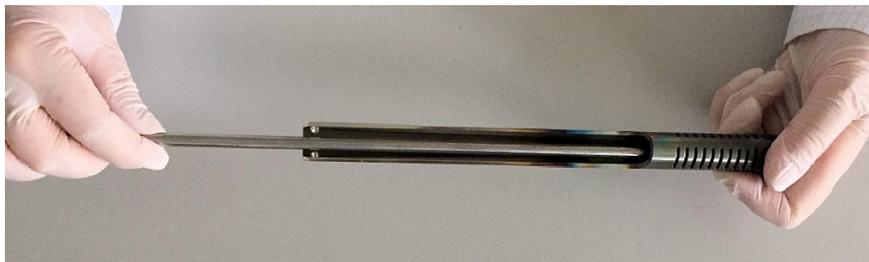
**Figure 14-2.** Removal of Ashes and Quartz Wool from the Crucible
