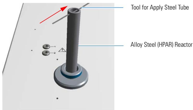
**Figure 9-6.** Introducing the Alloy Steel (HPAR) Reactor Into the Furnace
