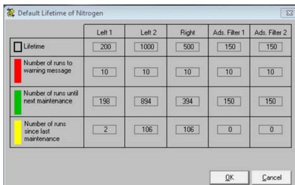
**Figure 13-2.** Maintenance: Example of Default Lifetime Condition
