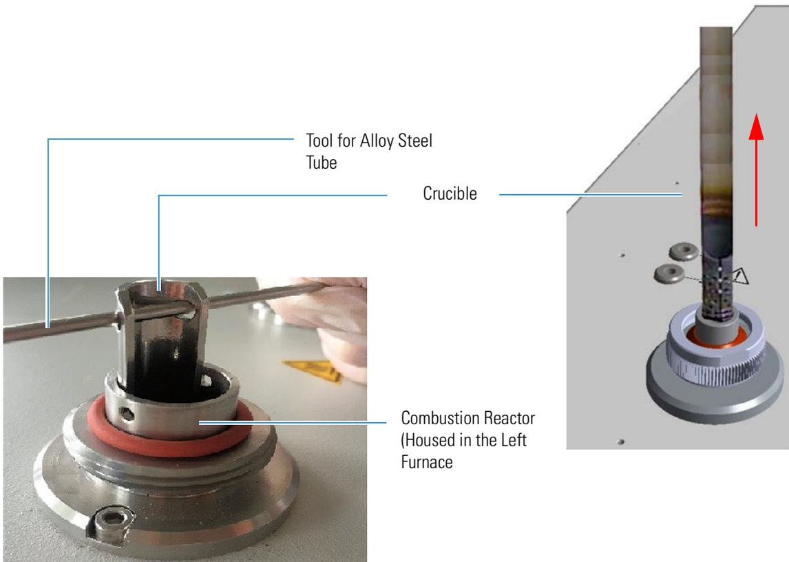
**Figure 9-18.** Removal of the Crucible
