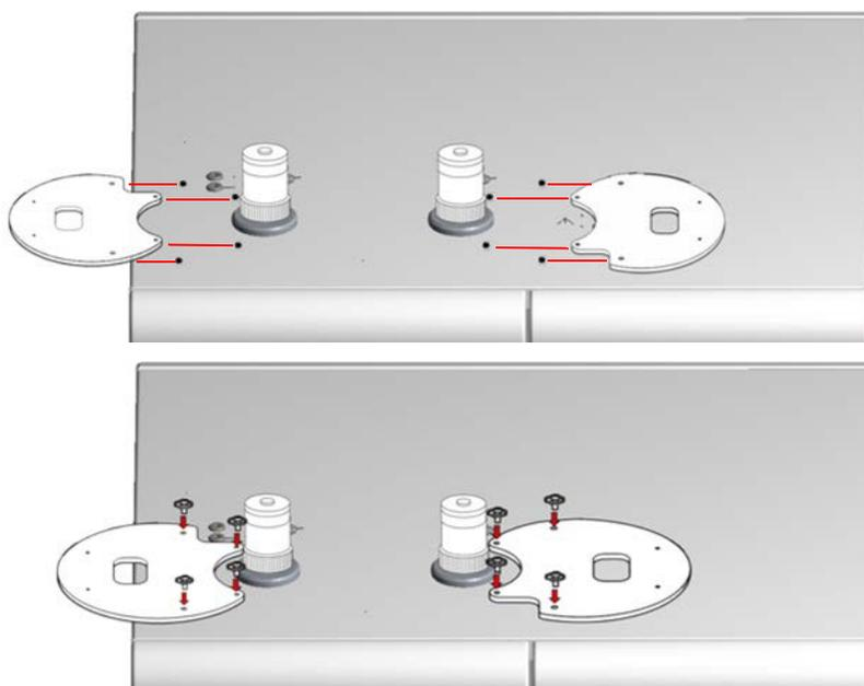
**Figure 7-6.** Mounting Support Bracket
