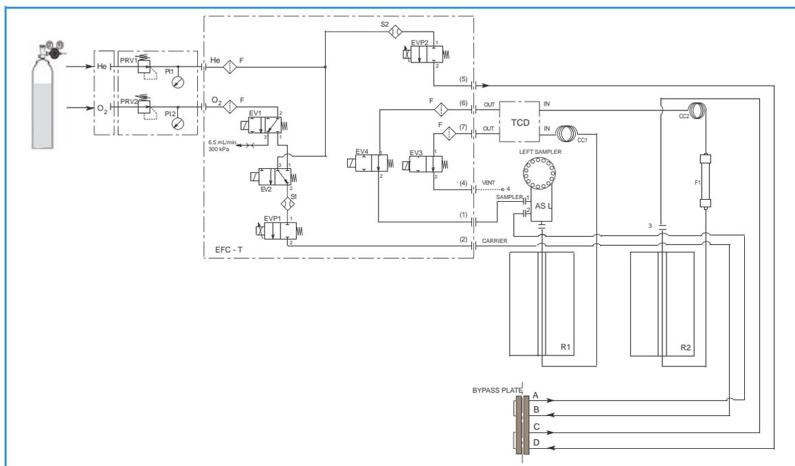
**Figure 4-11.** Instrument Parts Diagram and Pneumatic Diagram for CHNS/O Configuration with One Sampler
