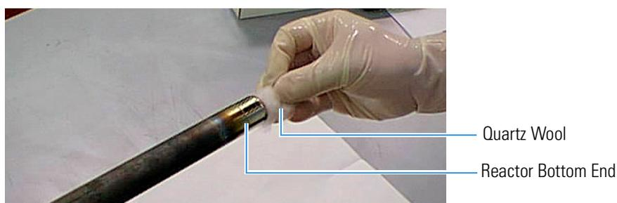
**Figure 8-5.** Introduction of Quartz Wool into the Bottom End of the Reactor
