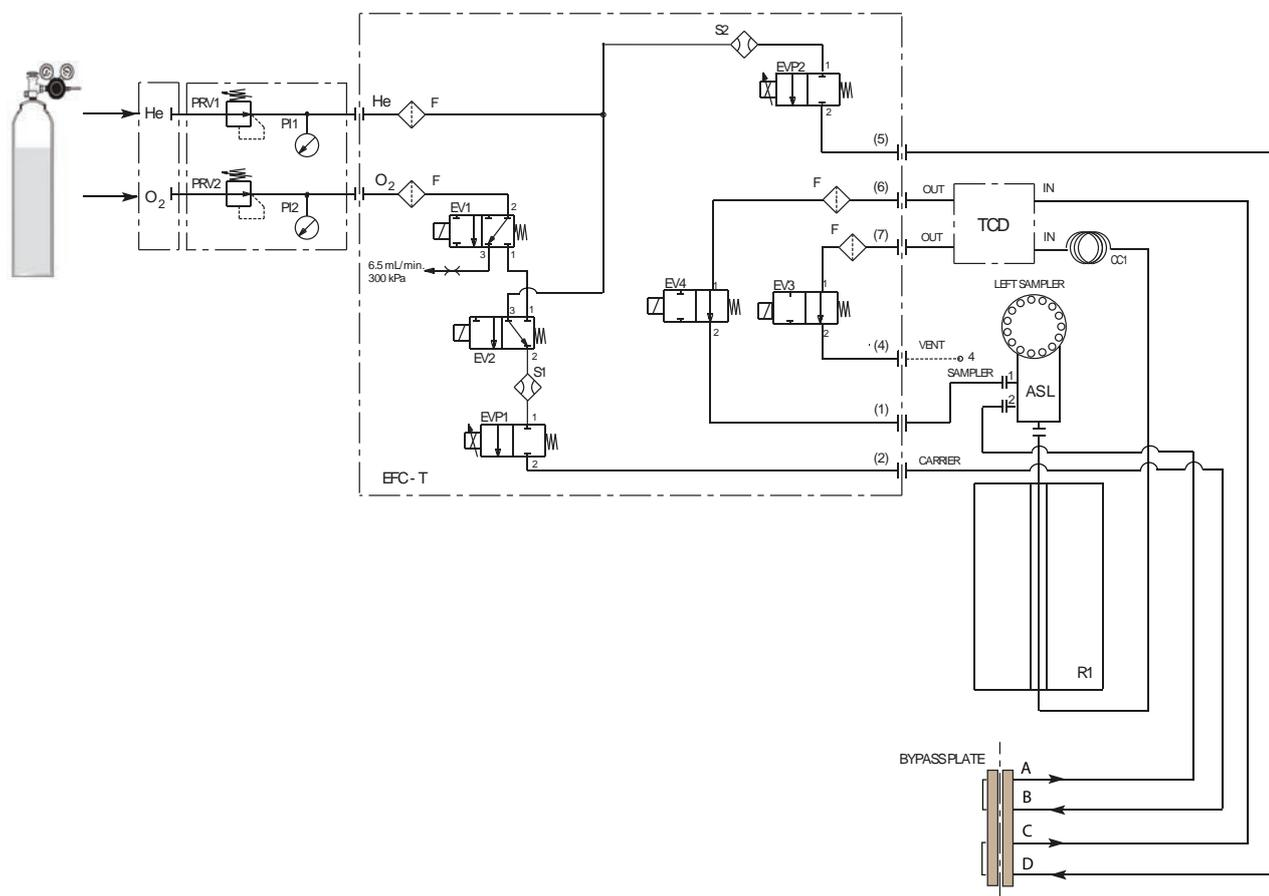
**Figure 4-9.** Instrument Parts Diagram and Pneumatic Diagram for CHNS Configuration
