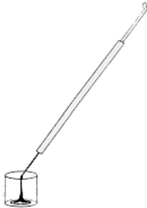
**Figure 10-11.** Introduction of a Viscous Sample into the Container
