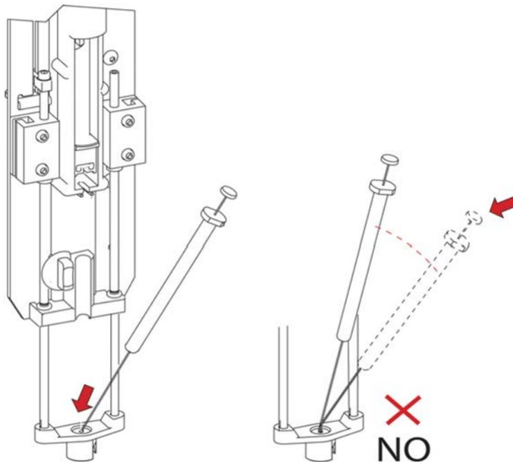
**Figure 7-15.** Syringe Installation (1)
