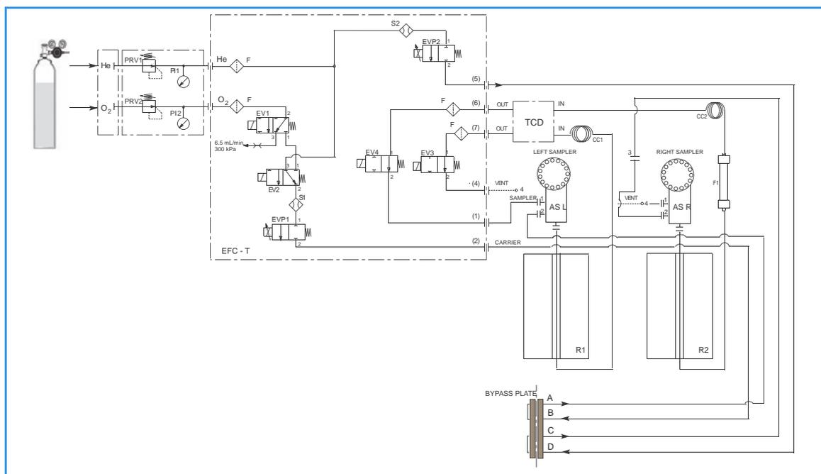
**Figure 4-6.** Instrument Parts Diagram and Pneumatic Diagram for CHN/O Configuration with Two Samplers
