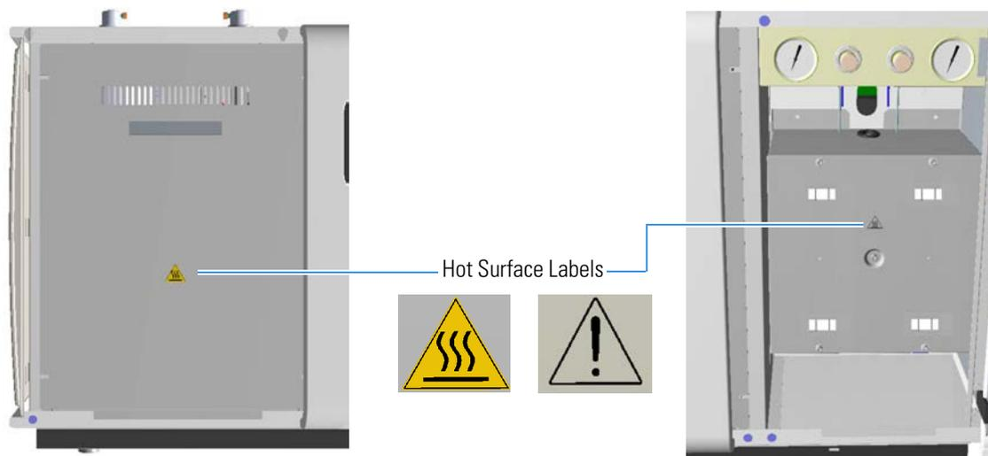
**Figure 2-2.** FlashSmart. Hot Surface labels
