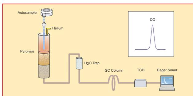
**Figure 4-18.** Schematic of O Configuration
