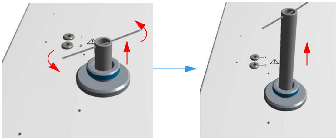
**Figure 9-20.** Removal of the Reactor
