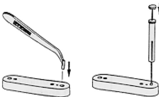
**Figure 10-8.** Housing for the Container and Sample Injection
