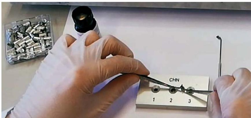
**Figure 10-6.** Preparation of the Container for Small Sample Quantities
