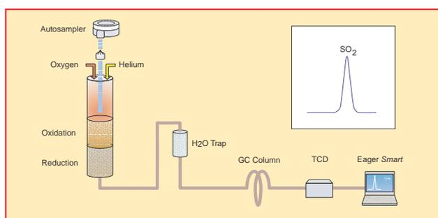
**Figure 4-16.** Schematic of S Configuration
