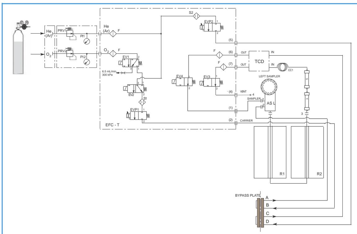
**Figure 4-27.** Instrument Parts Diagram and Pneumatic Diagram for N Lubricant, N Brew, and N/Protein Configurations
