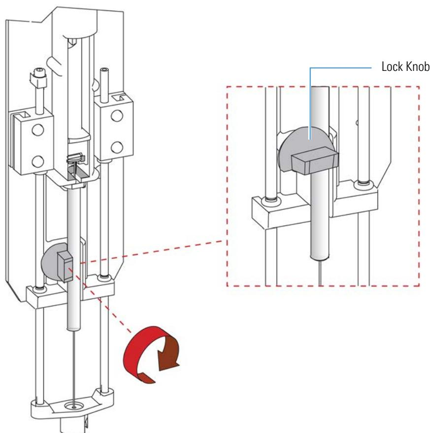
Figure 7-16. Syringe Installation (2)
