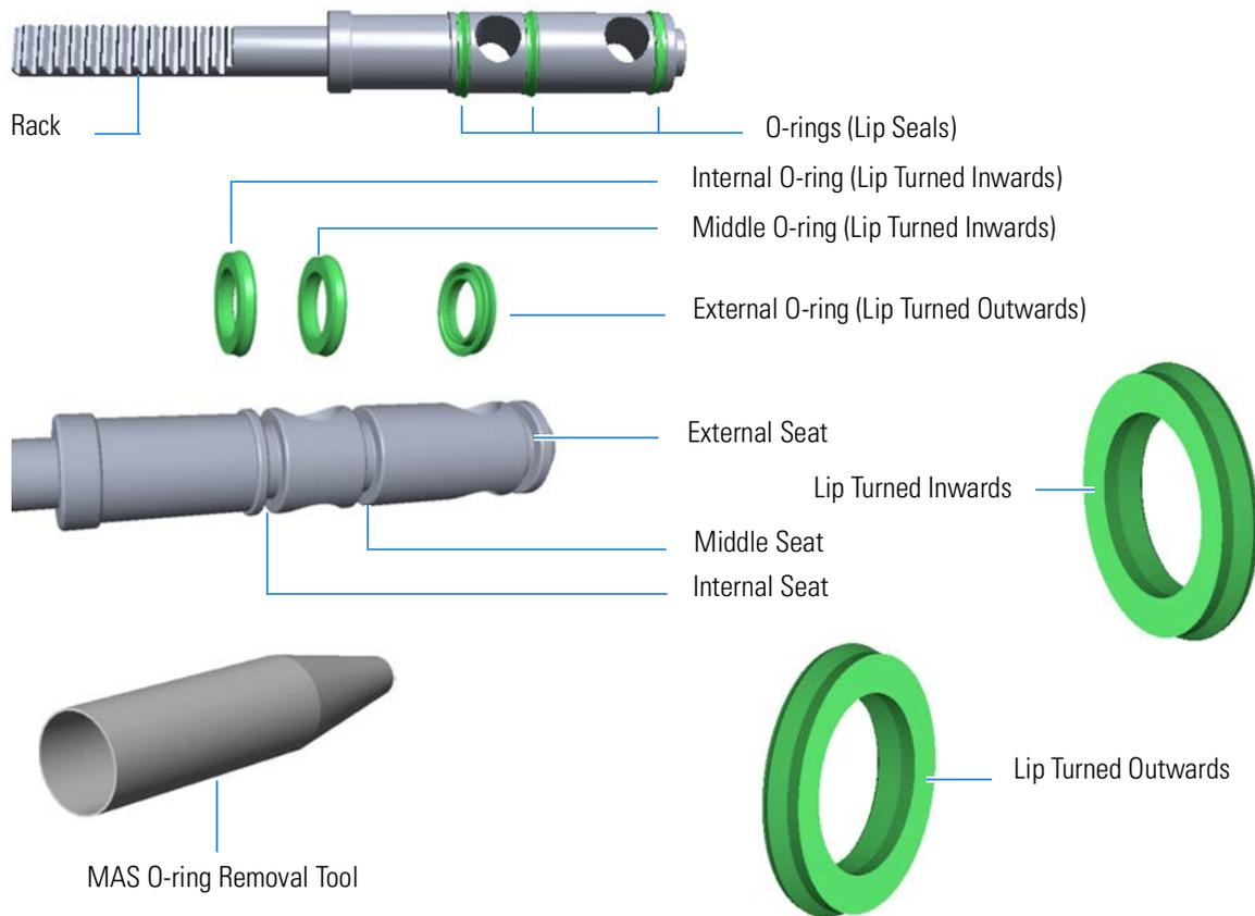
**Figure 14-15.** MAS O-ring removal tool
