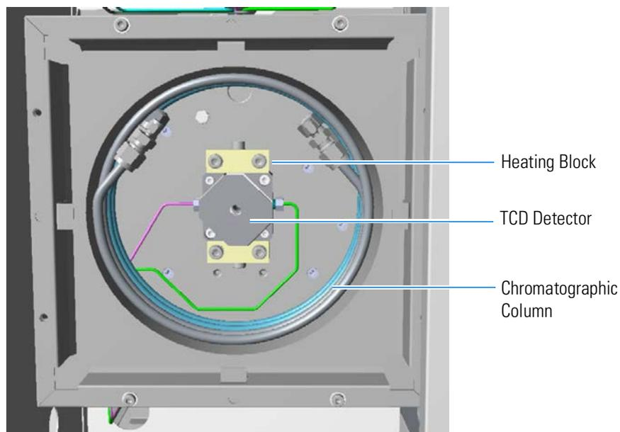
**Figure 14-5.** Compartment Housing the Chromatographic Column
