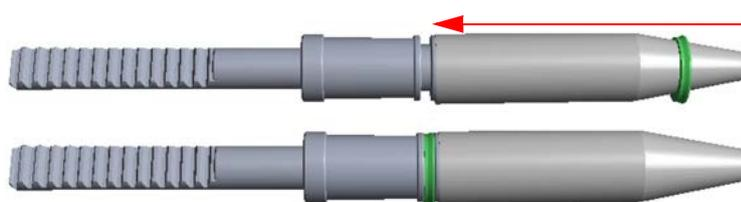
**Figure 14-17.** Moving the O-ring into the internal seat
