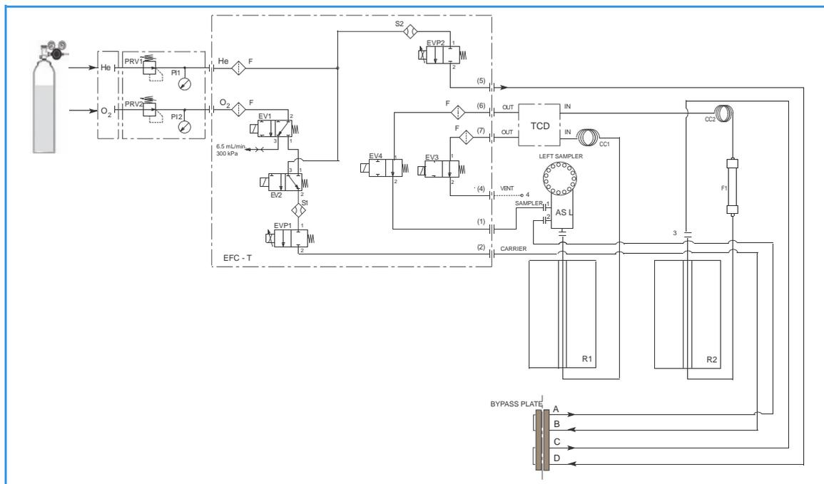
**Figure 4-5.** Instrument Parts Diagram and Pneumatic Diagram for CHN/O Configuration with One Sampler
