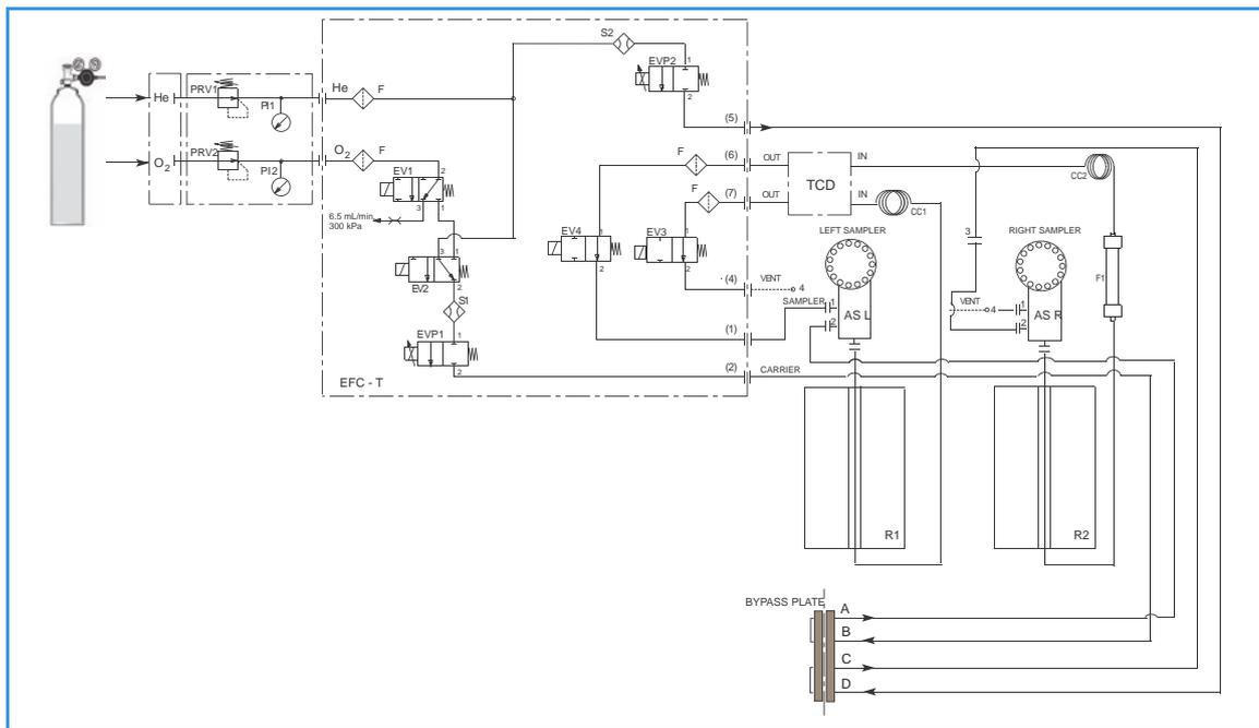
**Figure 4-12.** Instrument Parts Diagram and Pneumatic Diagram for CHNS/O Configuration with Two Samplers
