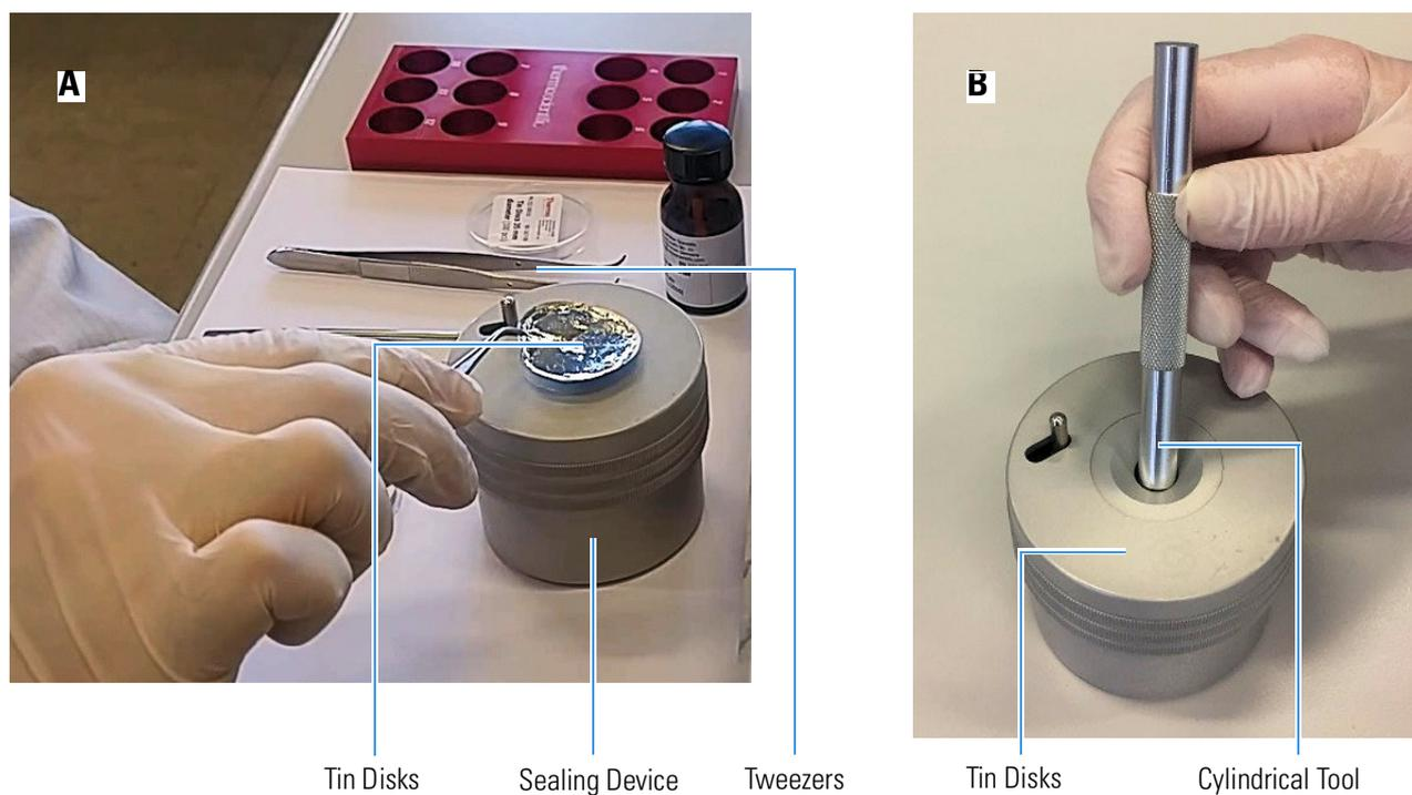
**Figure 10-2.** Preparation of the Tin Container (1)
