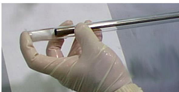
**Figure 8-2.** Compression of Quartz Wool into the Quartz Reactor
