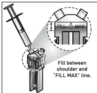
Check no air bubbles form in the cell - Tap the cell gently to dislodge any that form. Turn the cell upright and continue injecting slowly until the liquid reaches the fill area as shown. Remove syringe.
