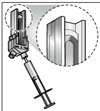
Invert the cell and slowly inject the sample from its syringe into the cell, filling the U tube to just over half way.
