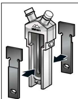
Fit the thermal contact plates as shown. These are stored in the pull out cuvette holder, located under the instrument.
