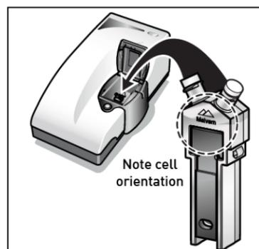
When inserting the cell, ensure that the Malvern logo faces towards the front of the instrument. Press down until the cell clicks into place. Before starting an experiment, ensure the software is set up to use the DTS1070 cell.
