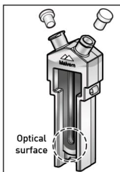
Fit one stopper firmly, the other one loosely, to avoid pressurisation of the cell. Remove any spillage from the electrodes.
