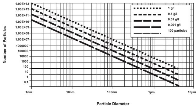
Figure 3.1 Number of particles per scattering volume for different concentrations
