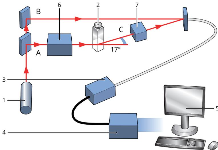
Figure 8.18 Zeta potential optical configuration
