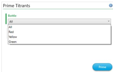
4. Select the cycles required and click the Prime button to begin the operation. Each cycle will pump the volume of the titrant tubes from the container.
