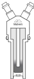
*Figure 3.2 Diffusion barrier in the folded capillary cell*
