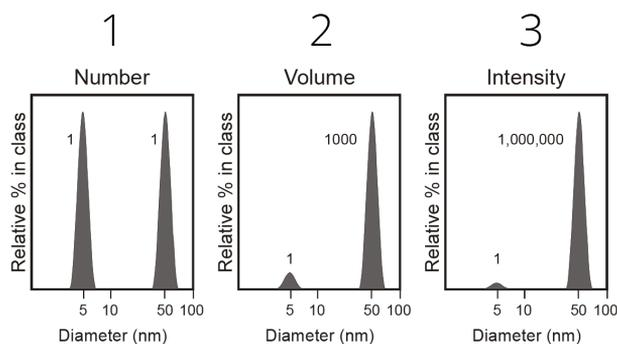
Figure 8.6 Number, volume and intensity graphs for the same measurement
