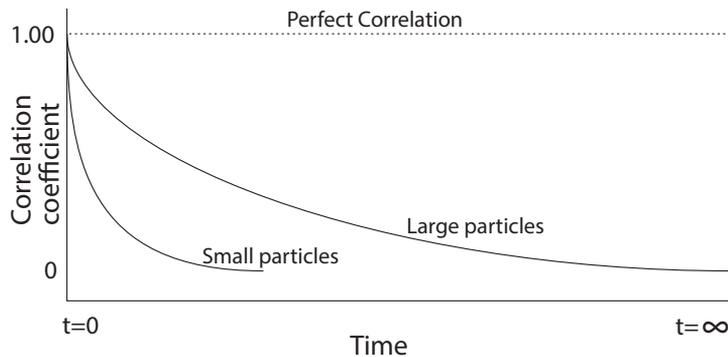
*Figure 8.4 Decay rate of correlation for large and small particles*
