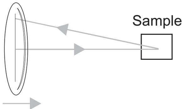
*Figure 8.10 Moving the lens towards the cuvette*
