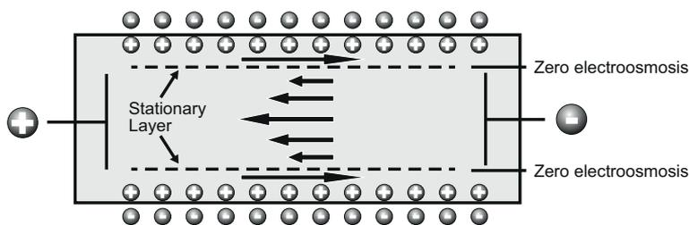
Figure 8.15 The stationary layer technique
