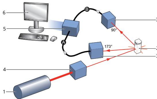
Figure 8.8 173°/90° measurement optics
