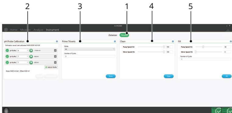
Figure 2.10 Titrator tab in the Instrument window
