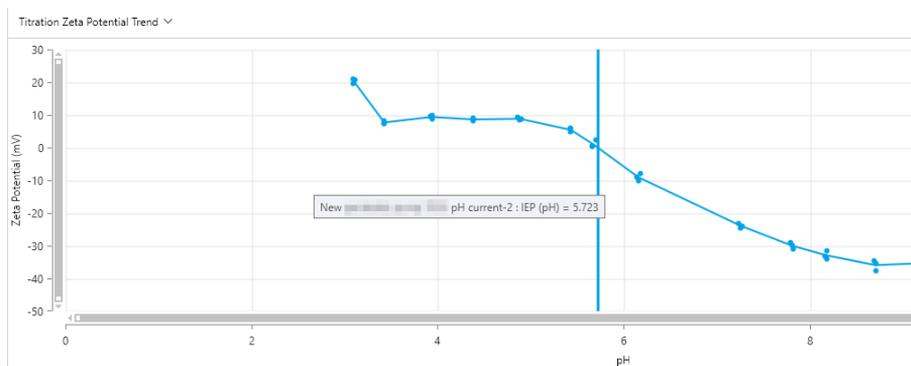
Figure 6.34 Displaying the IEP value
