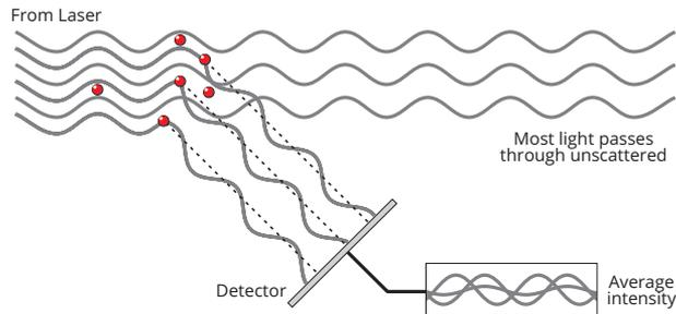
*Figure 8.1 Scattered light falling on the detector*
