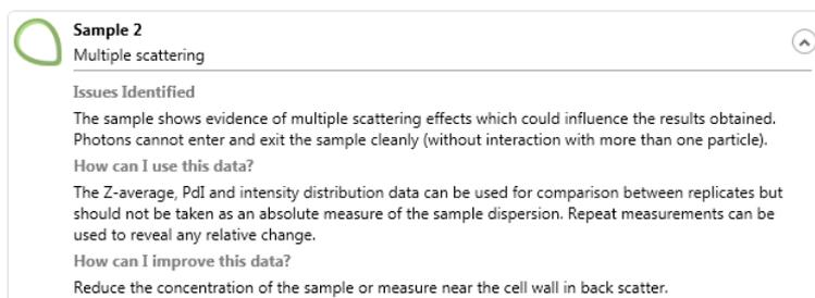
*Figure 7.4 Multiple scattering detected*
