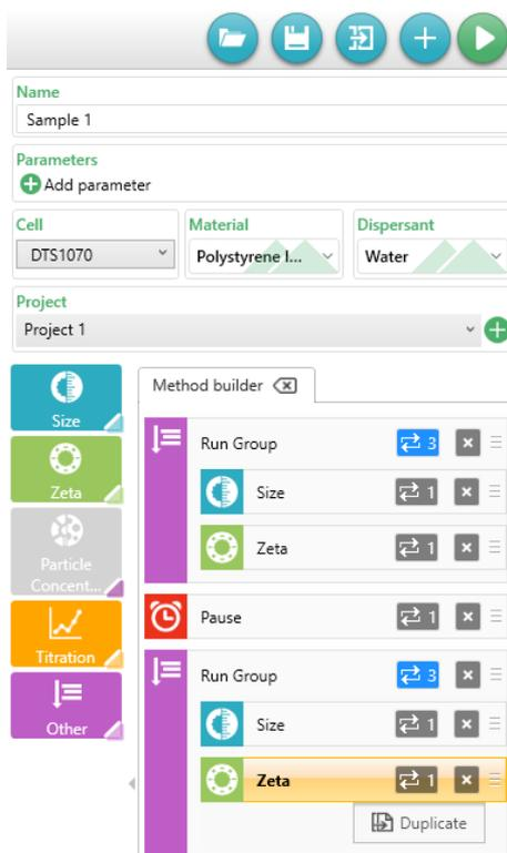
Figure 4.1 Example method in the Method builder
