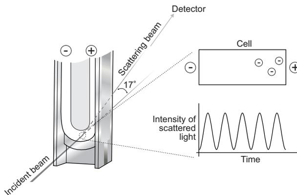
Figure 8.14 Laser Doppler Velocimetry
