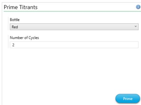
The screenshot shows a software window titled "Prime Titrants". Inside the window, there is a "Bottle" dropdown menu currently set to "Red". Below that is a "Number of Cycles" input field containing the number "2". At the bottom right of the window is a blue button labeled "Prime".
