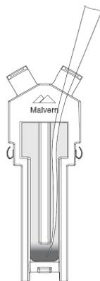
*Figure 3.3 Pipetting the slug of sample*
