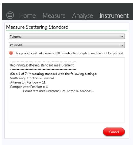
Figure 5.31 Measuring a scattering standard
