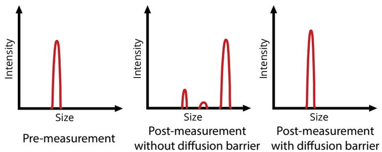
*Figure 3.4 Reduced aggregation visible after using diffusion barrier*
