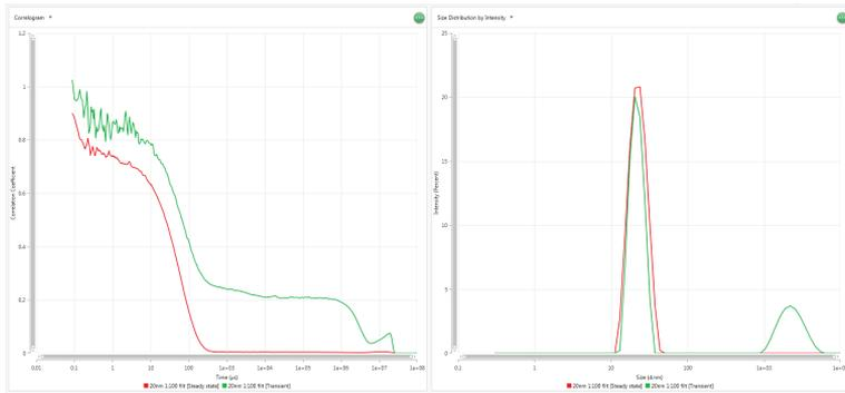
Figure 7.8 Overlaid transient (green) and steady state (red) data
